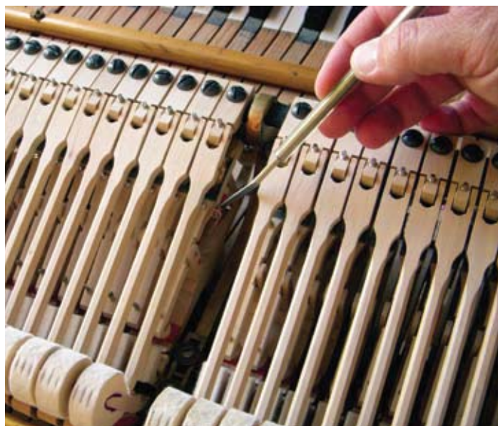
Photo 2: Working from the back of the action may be best for springs that wind off towards the bass.
