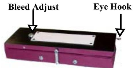
7. The rate of fallboard closure is set by a screw which controls the bleed rate. Turn clockwise to slow down, counter clockwise to speed up. We feel 10 seconds is optimal.
