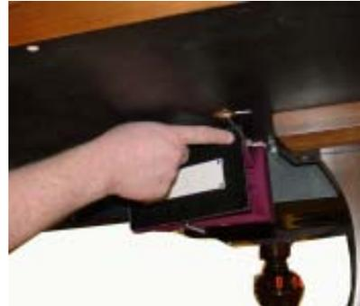
6. Thread cable through eye wire on pneumatic, apply felt washer and set collar. It may take a couple different settings of the set collar to find the desired (feel of catch) when closing key cover.
