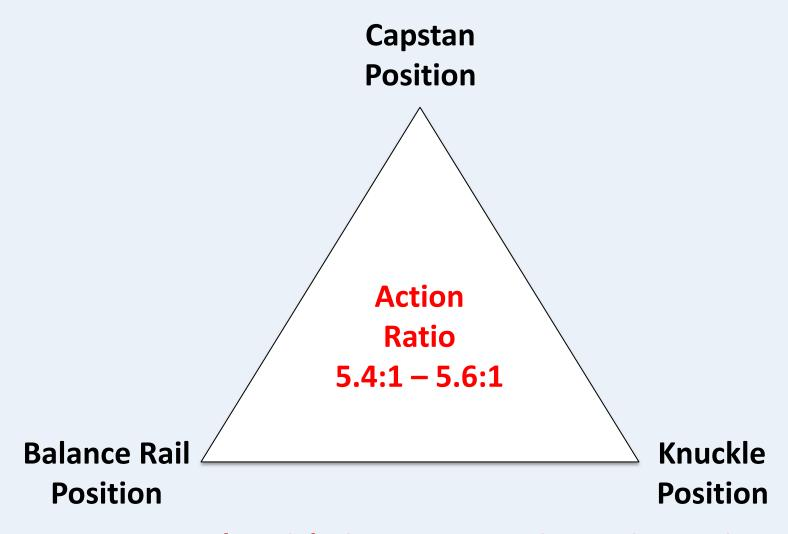
For touch weight issues, measuring Action Ratio 1<sup>st</sup> Most Important Measurement
