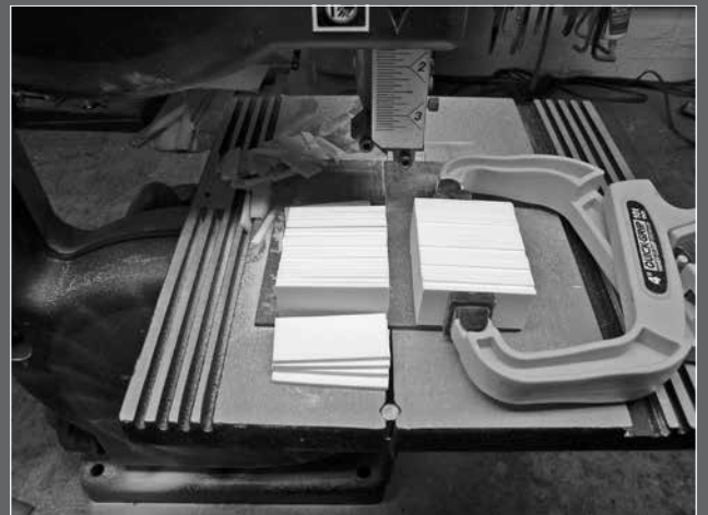
Once the pieces are grouped together for consistency, they are cut to length.
