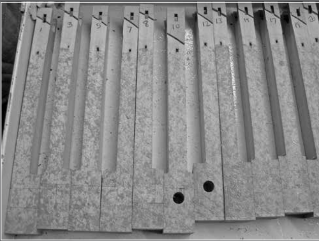
Plastic tops are removed to reveal that contact cement was used to apply them, and the key-stick surfaces not optimally prepared.
