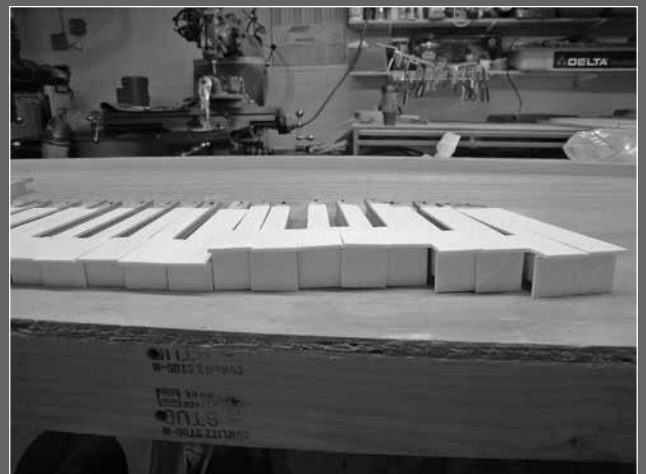
The new ivory key top in its rough-trimmed state, using a flush trim router bit.
