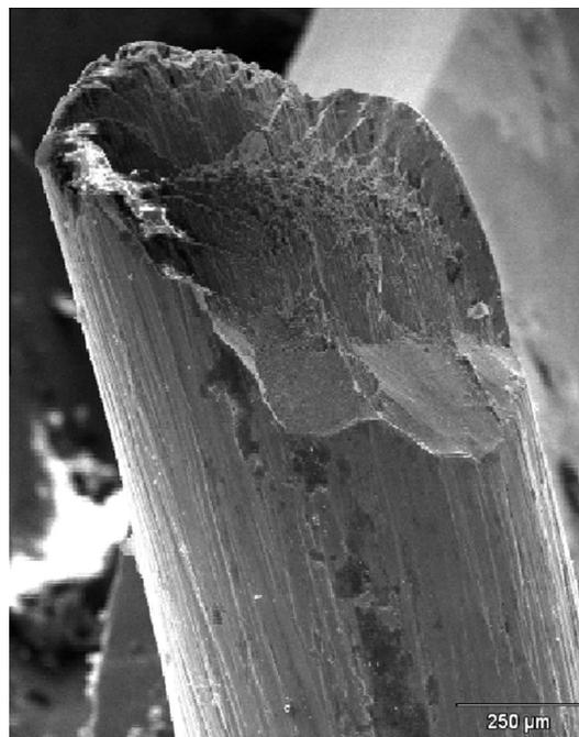
**Fig. 21.** Fatigue fracture of an acute string – SEM 80 $\times$ .
