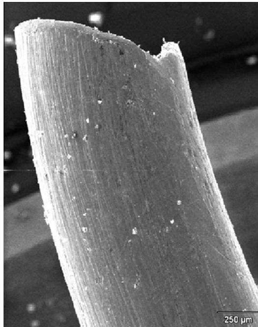
**Fig. 15.** Fatigue fracture of a lower bass string, SEM 60×.
