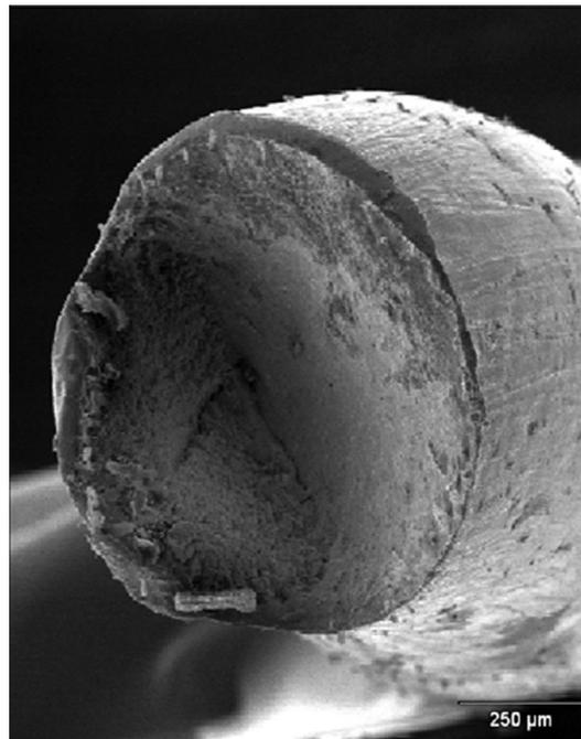
Fig. 16. Fatigue fracture of a lower bass string, SEM 80 $\times$ .
