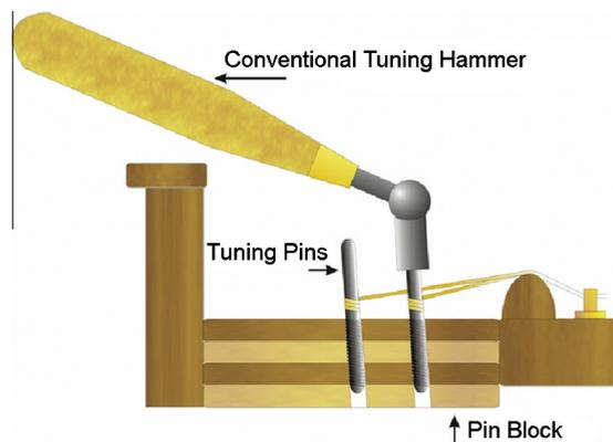
Fig. 25. Scheme of tuning pin-tuning hammer system.
