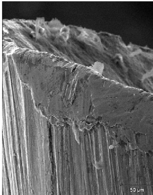
**Fig. 18.** Fracture surface, particular of a lower bass string, SEM 400 $\times$ .
