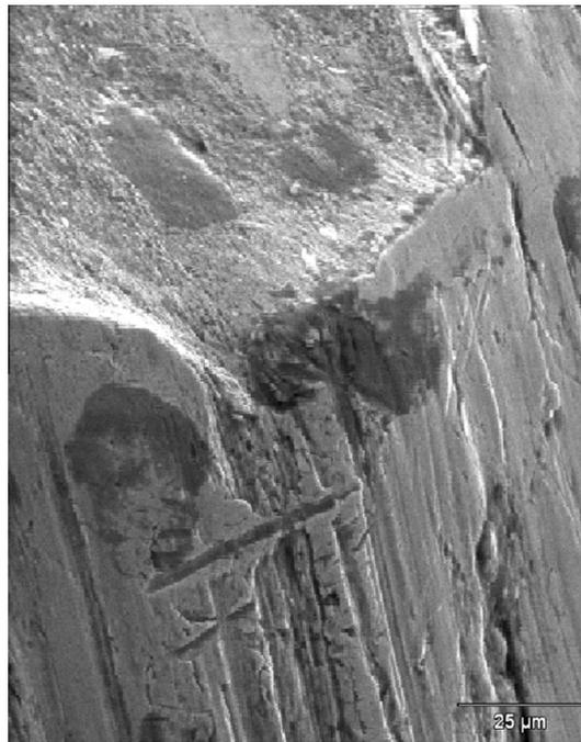
Fig. 22. Fatigue fracture of an acute string, magnification of the fracture surface – SEM 800 $\times$ .
