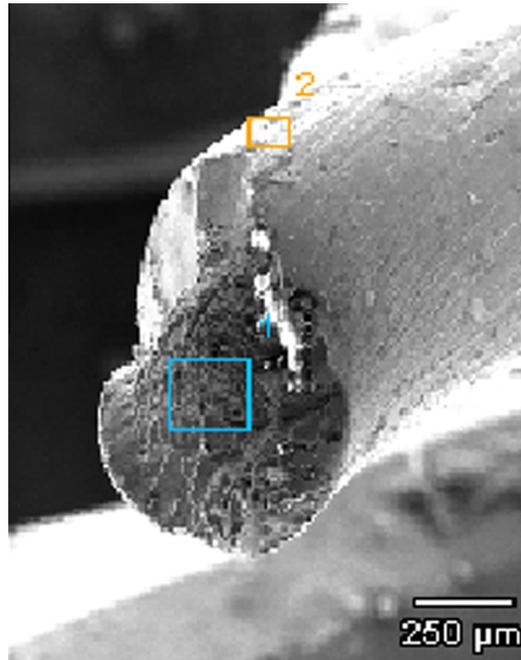
**Fig. 20.** Fatigue fracture of an acute string, EDS analysis area 70 $\times$ .
