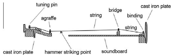
Fig. 6. Position of the string mounted on the cast iron plate.
