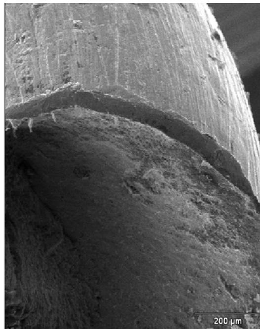
Fig. 17. Fatigue fracture of a lower bass string, SEM 120 $\times$ .
