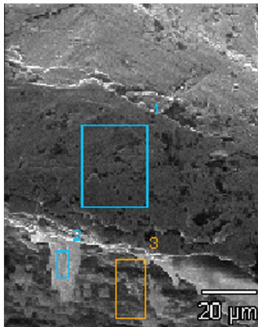
**Fig. 19.** Fatigue fracture of a lower bass string, EDS analysis area 100 $\times$ .
