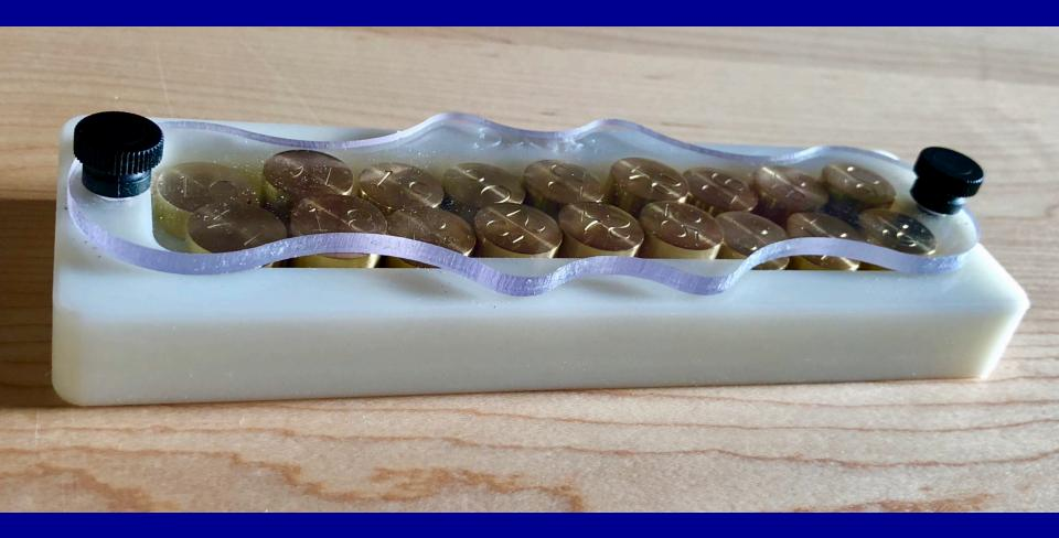
What is a Suitable **Balance Weight** For Most **Grand Actions?** 37g-39g BW (weights placed at front edge of key)
