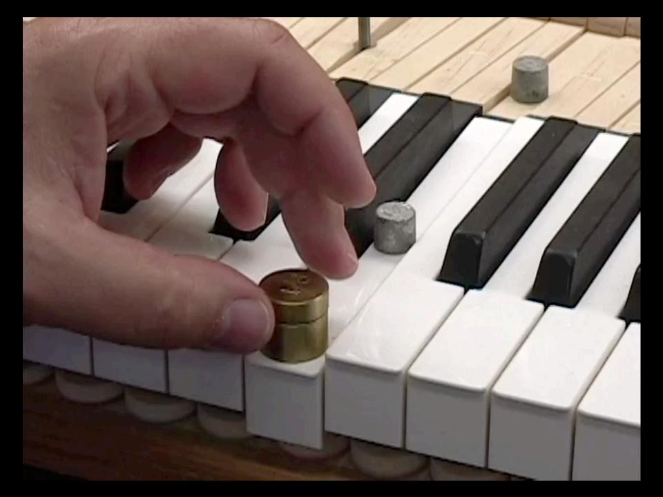
This Weigh-Off Method eliminates the problems created by target Downweight or Upweight numbers.
