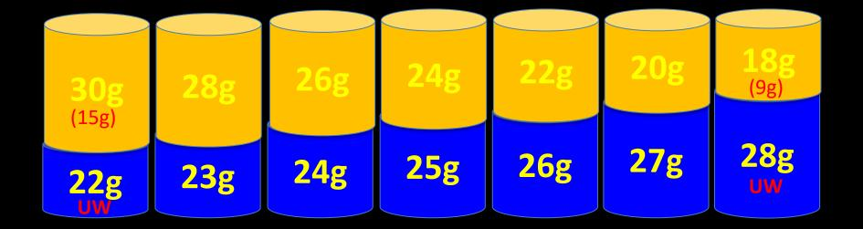
The Key Is Balanced When The "Slow" Key/Action Motion From The Total Stack Weight (DW) Is The Same As Upweight (UW)
