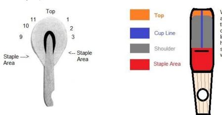
When the hammers are cut apart the released pressure on the outer edge of the hammer causes it to "cup" If you drew a line down the middle of the hammer you get the cup line, shown here in blue. This is where the needles go.
