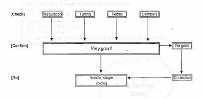
Important! Before voicing, make sure regulation, tuning, pedals and dampers are correct
