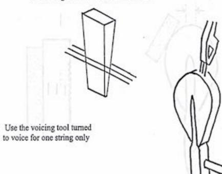
After needling, to settle the felt surface, tap the hammer with the handle end of the voicing tool.
