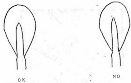
5. Side filing Used basically to remove needling marks
